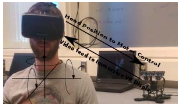
Figure 2: Diagram of head mounted Oculus Rift and camera on the gimbal. Position and angular rotation of the head mounted Oculus Rift is mapped to generate corresponding position and angular rotation in the camera on the gimbal. Video from the camera is mapped back to display in the Oculus Rift.
